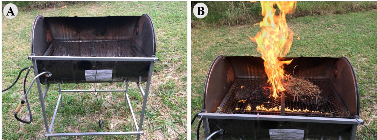
Figure S1: A) Equipment for flammability traits measurements built based on Jaureguiberry et al. 2011 . The device consisted of an 85 \times 60 cm barrel cut in half and arranged horizontally on four long metal legs. The barrel was open at the front and closed at the back for wind protection. Samples were arranged on a grill and placed horizontally to be heated by a burner located beneath the grill. B) An equipment views during the flammability traits measurements.
