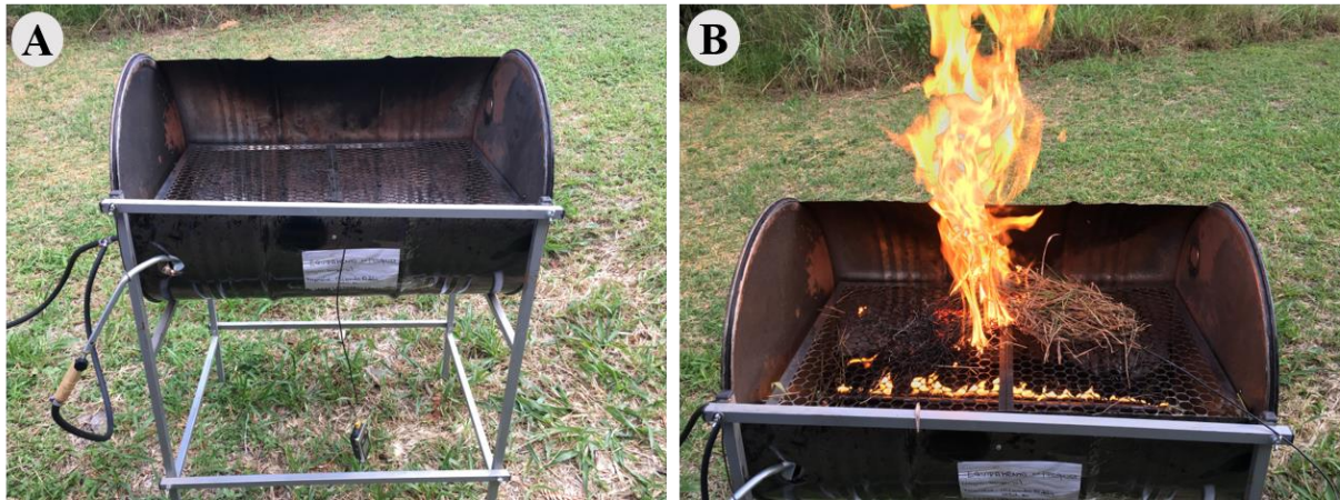
S1: A) Equipment for flammability traits measurements built based on Jaureguiberry et al. 2011 . The device consisted of an 85 \times 60 cm barrel cut in half and arranged horizontally on four long metal legs. The barrel was open at the front and closed at the back for wind protection. Samples were arranged on a grill and placed horizontally to be heated by a burner located beneath the grill. B) An equipment views during the flammability traits measurements.
