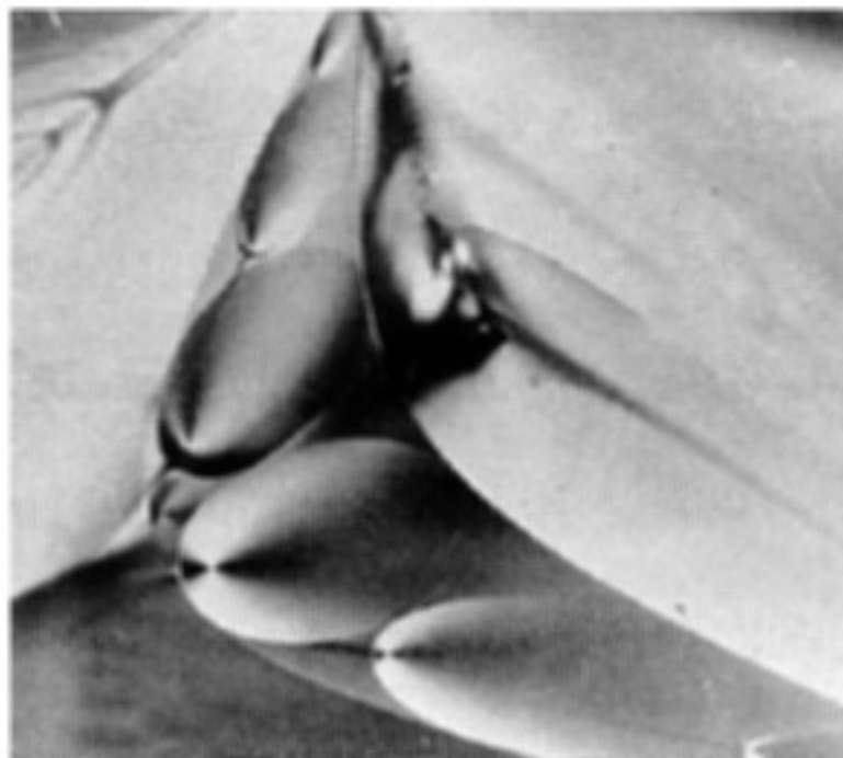
Figure 3.4: Focal conic domains: Pattern of ellipses and hyperbolas characteristic of the smectic-A microstructure. Image extracted from [10].
