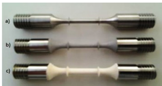
Figure 3. Photographs of the Ti-6Al-4V equiaxial alloy specimens with (a) no coating, (b) BC coating, and (c) TBC coating.
