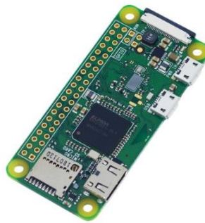
Figura 2: Placa Raspberry Pi Zero W
