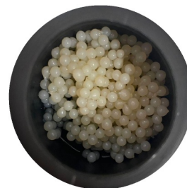
FIGURE 2 | Mycogenic silver nanoparticles (AgNPs) encapsulated in calcium alginate (CA) beads with a medium diameter of 4 mm.
