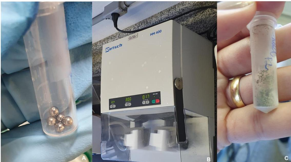
**Figure 1.** Egg's maceration process. A) For each sample, were used five spheres; B) ball mill; C) Fine powder of eggs.
