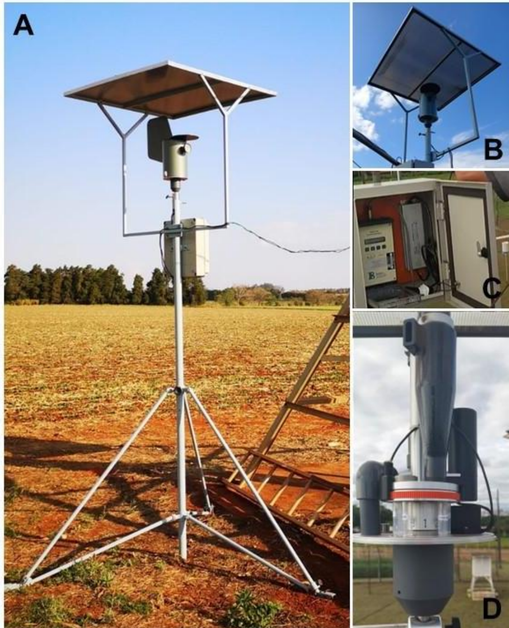
Figure 1 - (A) High-volume cyclone air sampler from Agri Samplers Ltd. (UK), installed in Londrina, PR, operating at the IDR Paraná Experimental Station (Institute of Rural Development of Paraná); (B) Front view of the sampler unit; (C) Control panel through which the sampler parameters are set; and (D) Details of the open spore sampler unit.
