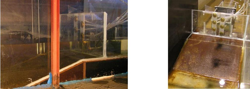
Figure 3: Physical breakwater model in the flume with position of the pressure sensors.
