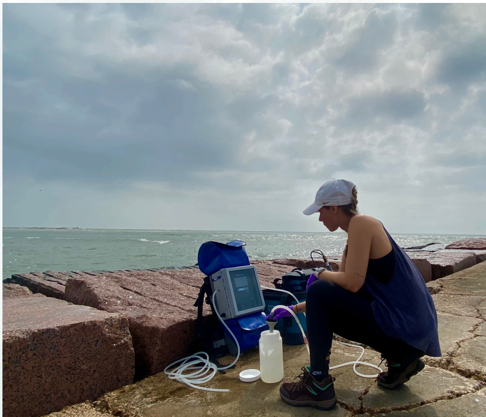
Figure 1. Collection and filtration of water samples for environmental DNA (eDNA) analysis using a Smith-Root eDNA Sampler ( https://www.smith-root.com/edna/edna-sampler ). Image credits: Ingrid Bunholi and Mary Finch.
