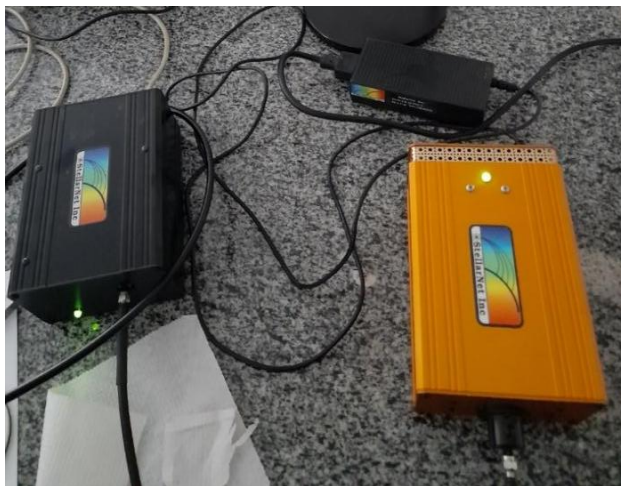
Figure 3.7: StellarNet fiber optic spectrometer coupled to UV-VIS Light Source. Source: own authorship
