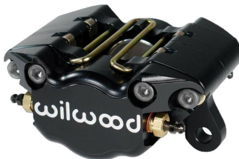
Figura 3.5 – Pinça de freio Wilwood Dynapro Single
