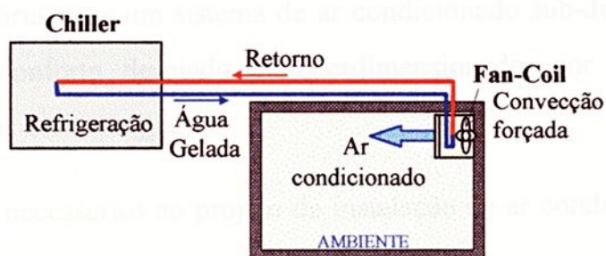
CHILLER E FAN-COIL
