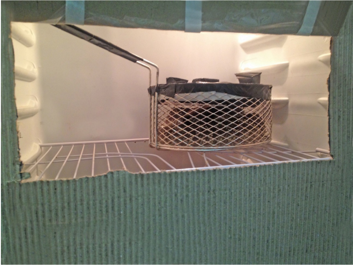
Figure 12. A rattlesnake inside the wired mesh container used to verify the critical thermal limits (i.e., to turn snakes on their dorsum; see text for details) arranged inside a BOD climatic chamber.
