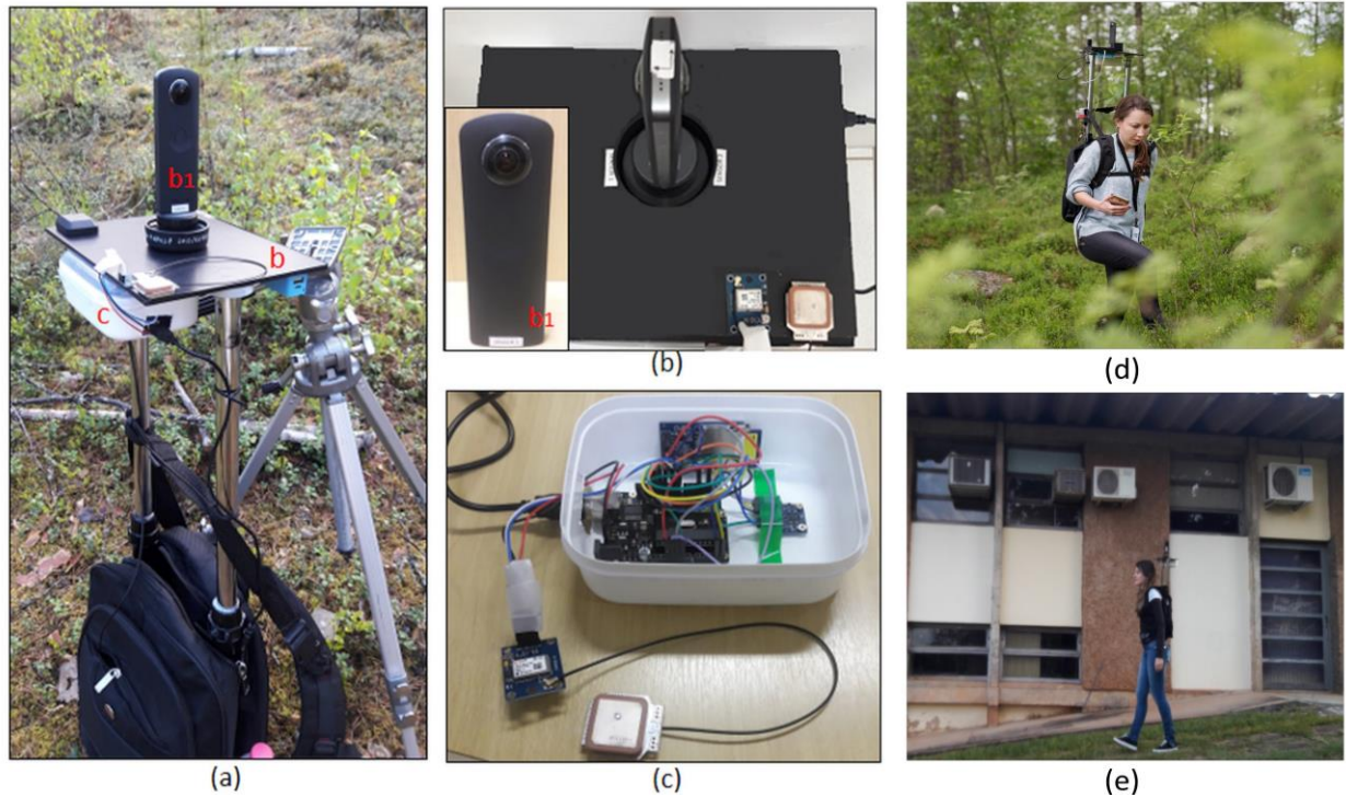
Figure 1. Personal Mobile Terrestrial System (PMTS): (a) Backpack platform structure and PMTS sensors; (b) Top view of platform with the omnidirectional camera and GPS receiver; (c) Navigation sensors; (d) Example of an operator carrying the PMTS inside a boreal forest site and (e) urban area.
