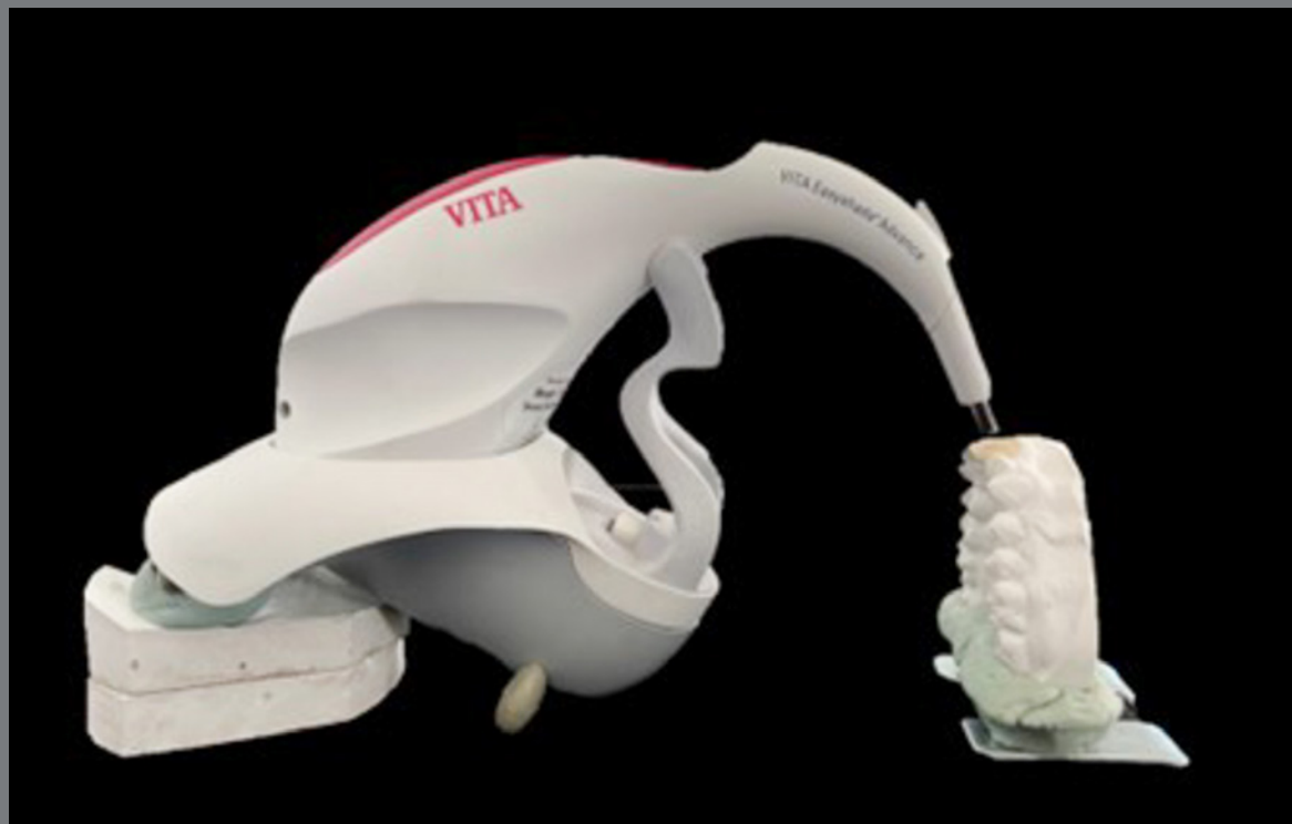
Figure 2: VITA EasyShade® Advance digital spectrophotometer.
