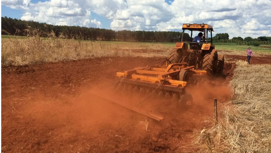
Figura 8 - Preparo convencional do solo com grade pesada - GPC: Preparo secundário com grade de 32 discos com diâmetro de 22" para destorroamento do solo, safra de verão 2018/2019. Figure 8 - Conventional tillage with a heavy harrow - GPC: Secondary tillage with a 32-disk harrow with a 22 "diameter for soil removal, 2018/2019 summer harvest.
