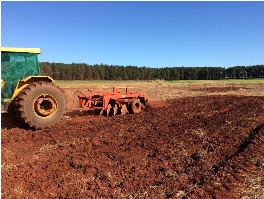
Figura 9 - Preparo convencional do solo com grade pesada - GPC: Segunda operação de grade pesada efetuado com grade pesada de 14 discos recortados com diâmetro de 32" x 9,0 mm, safra de verão 2018/2019. Figure 9 - Conventional soil preparation with heavy harrow - GPC: Second heavy harrow operation carried out with a heavy harrow of 14 cut-out discs with a diameter of 32 "x 9.0 mm, summer harvest 2018/2019.
