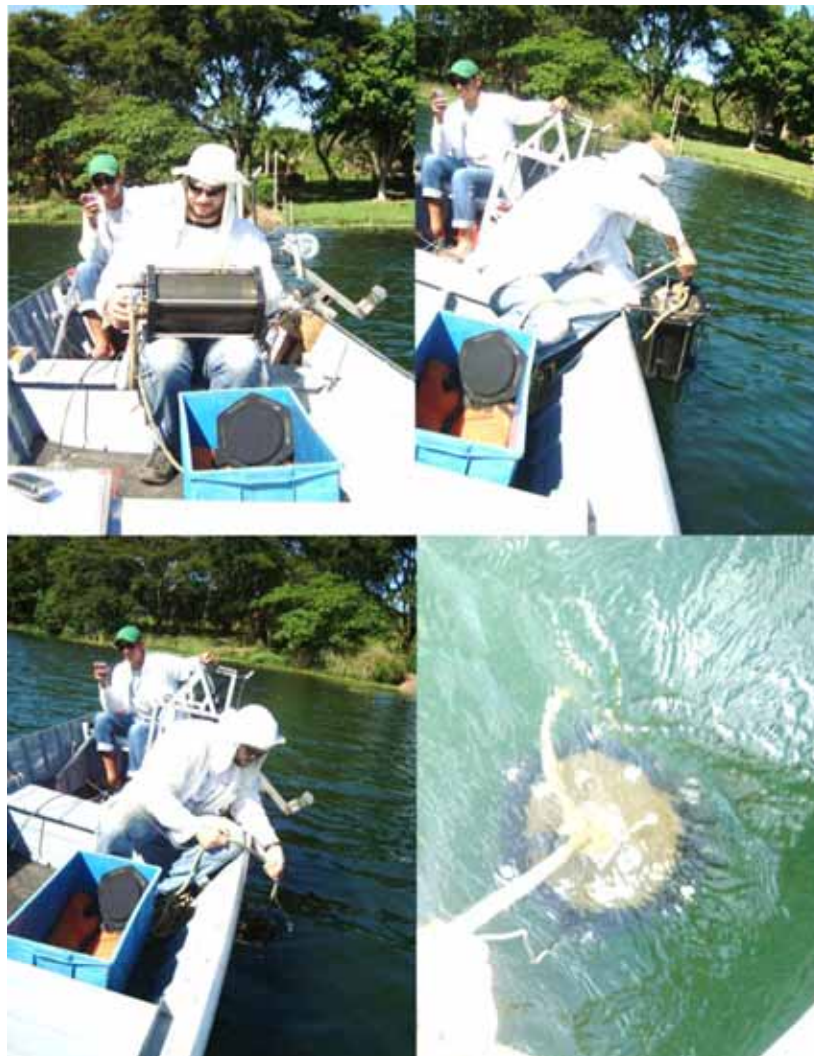
Figure 15 – Backscattering coefficient measured by HydroScat equipment.
