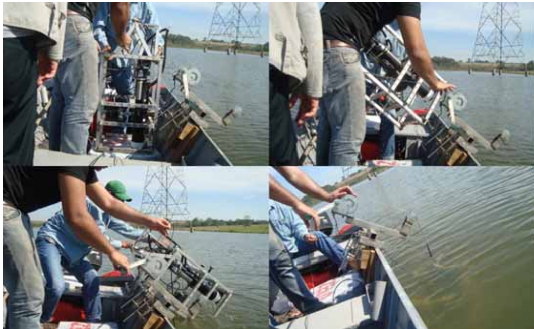
Figure 14 – The AC-S measuring the absorption and attenuation coefficient.
