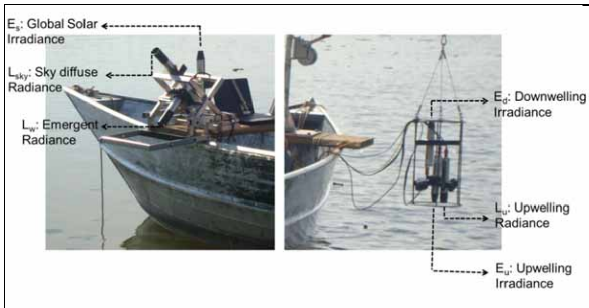
Figure 12 – Radiometers (RAMSES/TriOS) used to obtain hyperspectral data.
