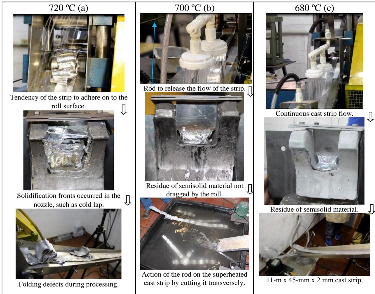
Fig. 1. Production of cast metal strips employing single-roll processing.
