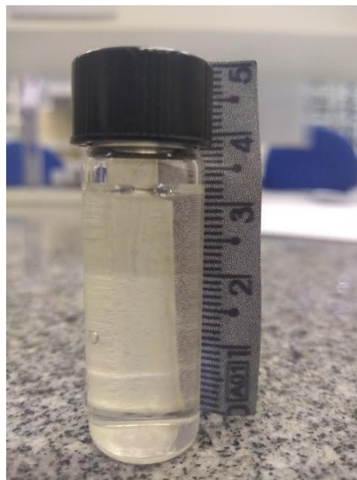
Figure 33 - Round flask with 4 mL water and a printed ruler attached, in order to measure water vapor transmission rate through bioplastic, which is attached to the lid opening
