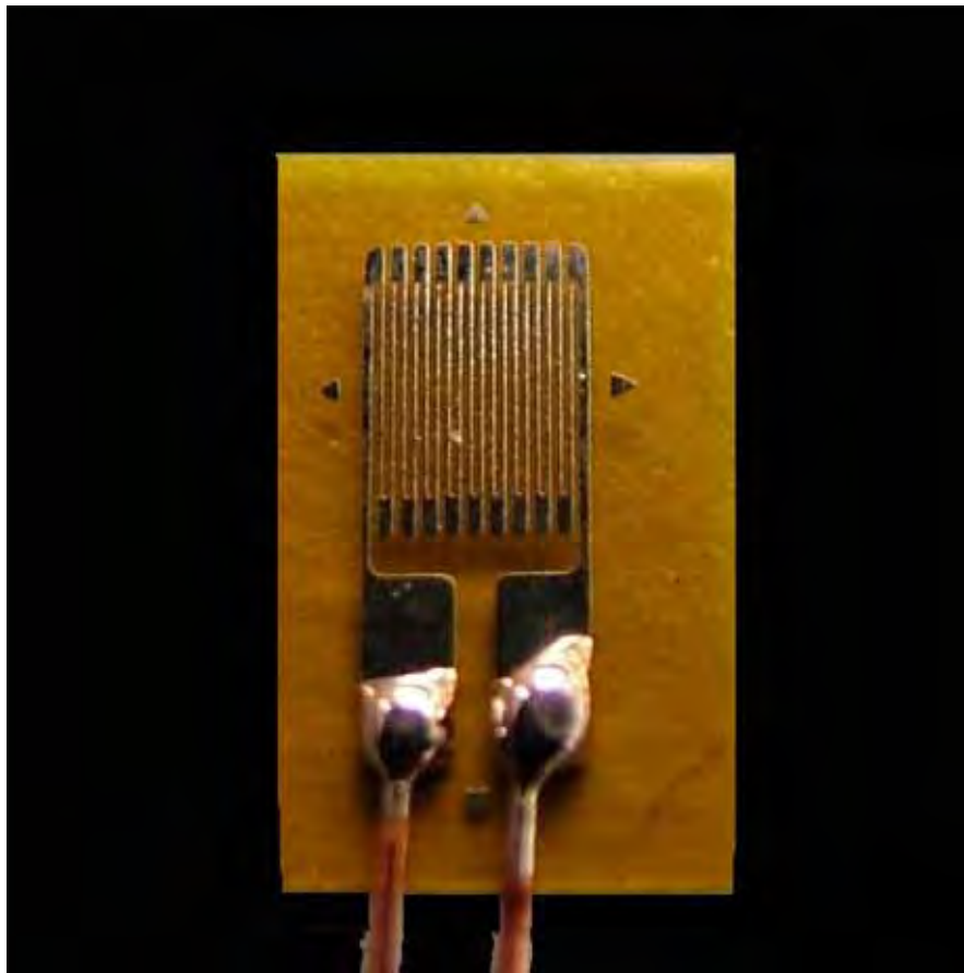
FIGURA 4 – Strain gauge modelo PA-06-062AB-120L (Excel Sensores Ltda)
