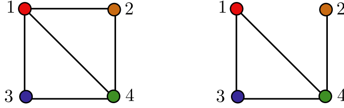
Figure 5.3: One edge irreducible graph. We show on the left a one edge irreducible graph and on the right a non irreducible one. If we cut the 2 – 4 bridge of the right graph we get a disconnected graph.
