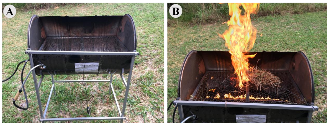
Figure SI 1: A) Equipment for flammability components measurements built based on Jaureguiberry et al. 2011 . The device consisted of an 85 × 60 cm barrel cut in half and arranged horizontally on four long metal legs. The barrel was open at the front and closed at the back for wind protection. Samples were arranged on a grill and placed horizontally to be heated by a burner located beneath the grill. B) An equipment views during the flammability measurements.
