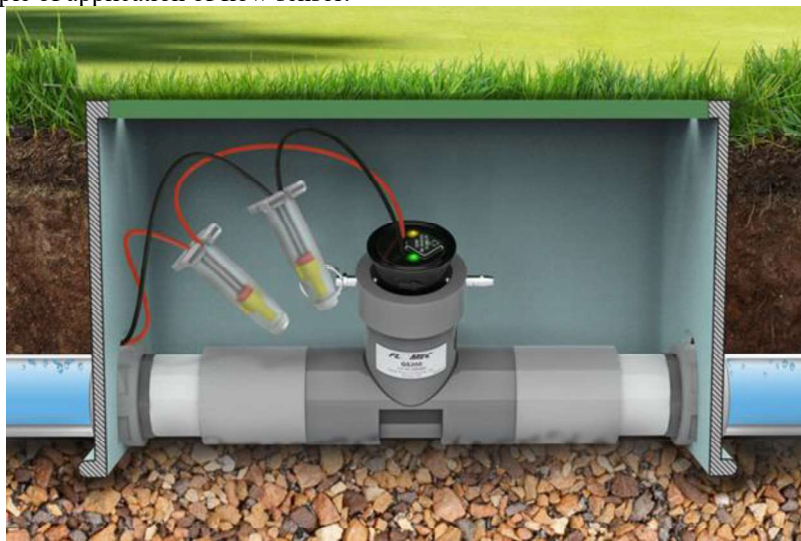
Figure 1.8 - Example of application of flow sensor.
