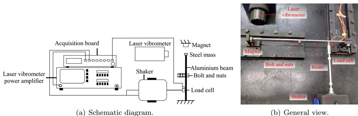
**Figure 1.** Experimental setup of the magneto-elastic system.
