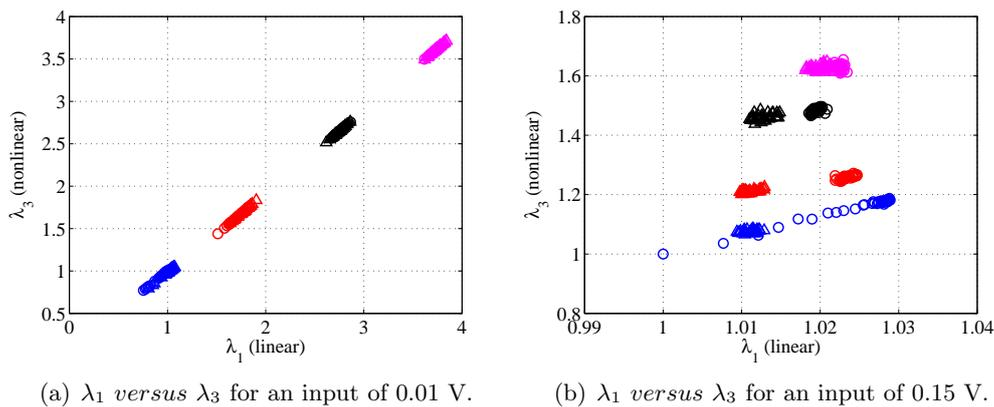
**Figure 8.** Comparison between the linear index  $\lambda_1$  and the nonlinear index  $\lambda_3$ . **Blue** is the reference state with 4 nuts, **Red** is the case with 3 nuts, **Black** represents the case with 2 nuts and **Purple** is the case with 1 nut. Circles  $\circ$  represent the case where the damage is being applied and triangles  $\triangle$  represent the repaired cases.
