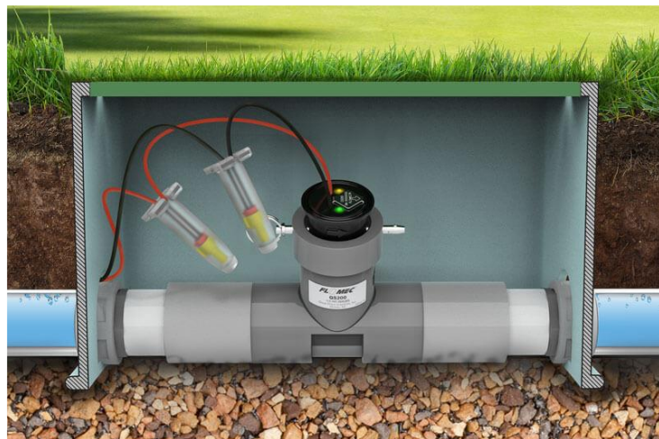
Figure 4 – Example for the application of flow sensors in a buried water pipe.
