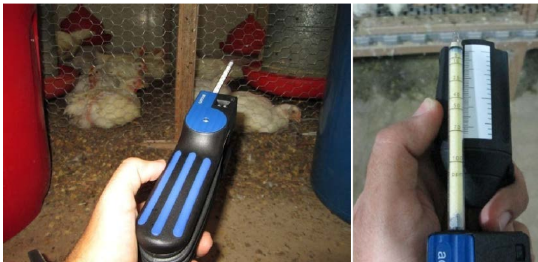
Figura 4 – a) Bomba detectora de gases Dräger Accuro®, b) Tubete reagente
