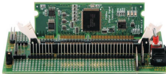
Figure 65 – DSP kit with TMS320F28335 controlCARD. Adapted from (TI, 2011).
