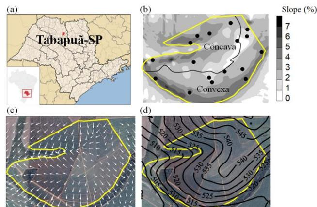
FIGURE 1. Location of the area close to the Turvo river (a), slope map and 17 observation points for simulated rainfall information collection (b), surface water flow simulation (c), and planialtimetric map with altitude in meters (d). Adapted from Ibiapina (2015).
