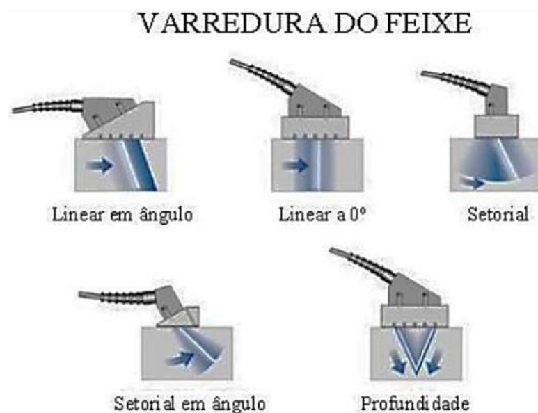
Figura 29 - Formas de varredura com o Phased Array.
