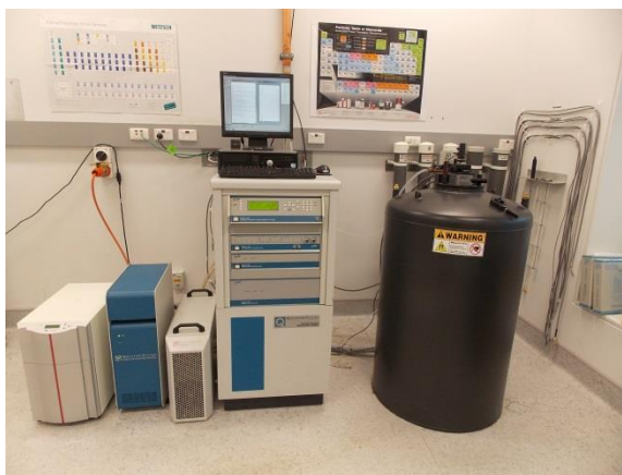
Figura 3.15 – Physical Property Measurement System (PPMS), modelo 6000, com AC transport controller, modelo 7100. (ISEM, University of Wollongong).
