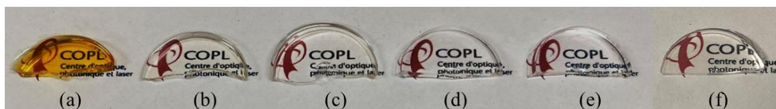
Fig. 3.3. Aluminophosphosilicate samples heat-treated at different temperatures (a) gel dried at 80 °C, (b) 550 °C, (c) 600 °C, (d) 700 °C, (e) 800 °C and (f) 900 °C (under vacuum).
