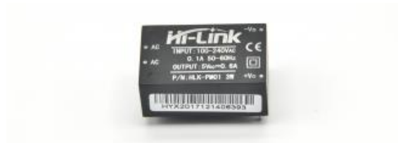
Figura 14 – Módulo Conversor AC-DC HLK-PM01
