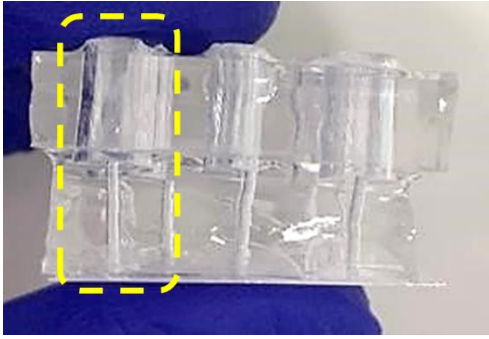
Figure 5. Alignment of master mold and reservoir mold after plasma bonding. The second step of plasma bonding requires the alignment of both molds. On the top is the reservoir mold aligned with the master mold on the bottom.
