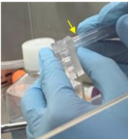
Figure 6. Type IV Matrigel vacuuming. A square-shaped piece of PDMS with a single hole punch on top of the reservoir mold. A pipette tip (connected to the vacuum) inserted in the punch aligned with the AMC chamber reservoir.
