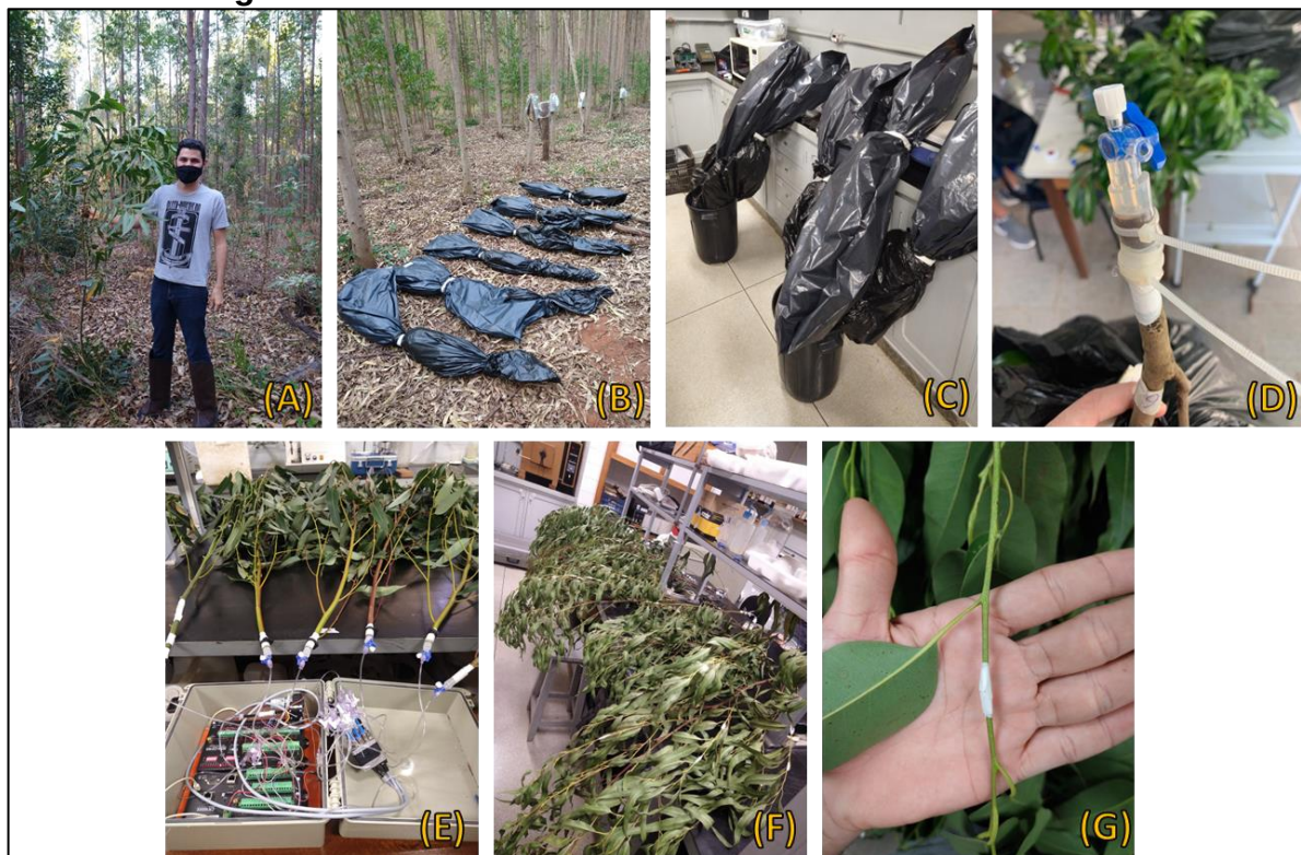
Figure 2 – Workflow of the Pneumatron measurements
