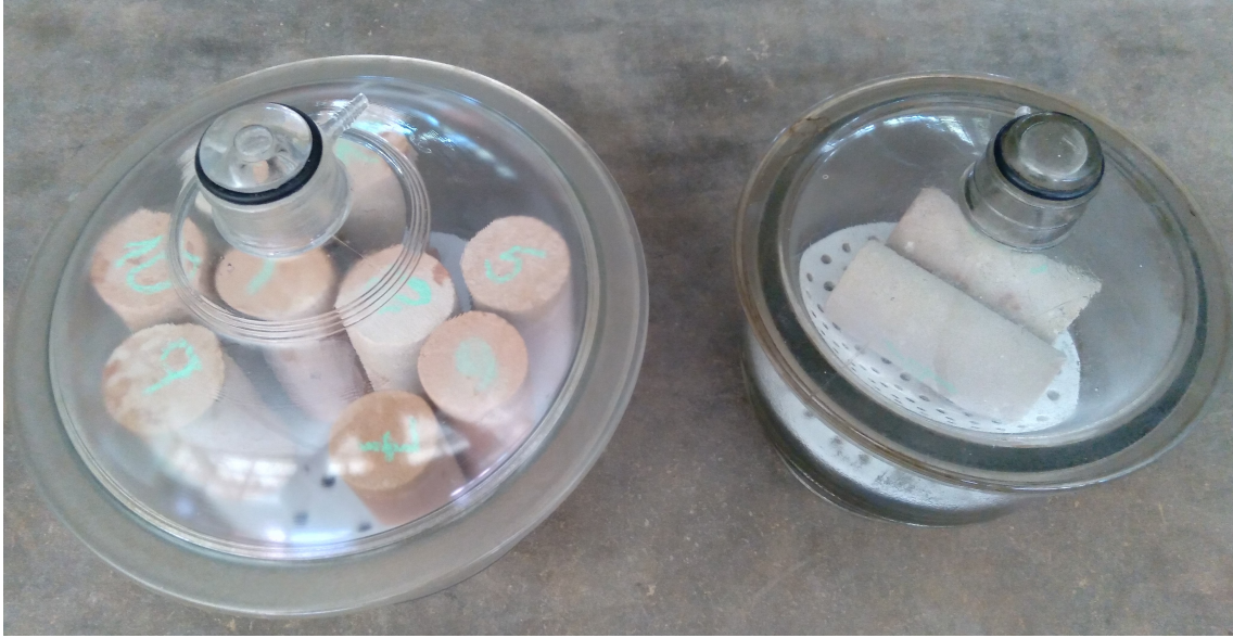
Figure 2.23: Cooling the specimens to room temperature in a desiccator.
