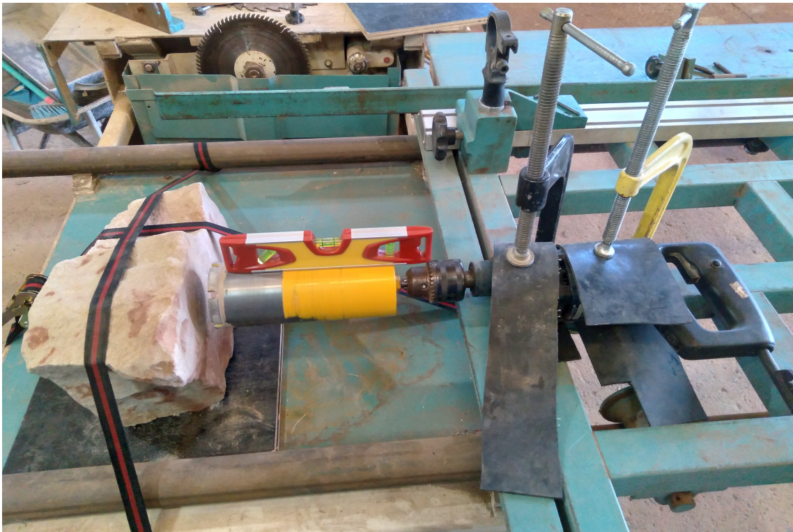
Figure 3.7: Assembly of the diamond hollow core drill used to remove cylindrical rock samples.
