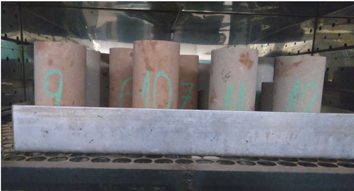
Figure 2.22: Pre-drying the specimens in the oven.
