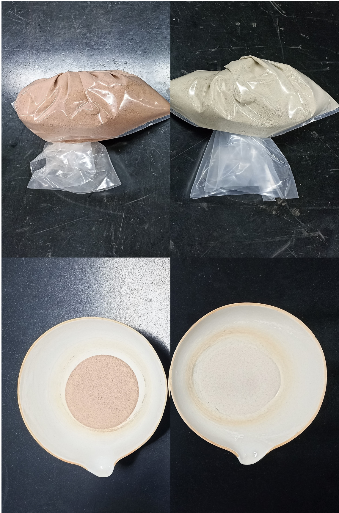
Figure 2.7: Preparation of the samples selected by predominant color for the particle size test.
