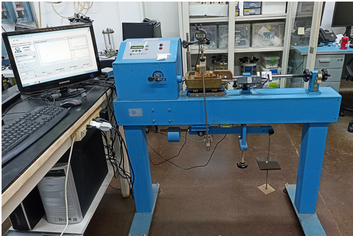
Figure 2.30: Direct shear machine and data acquisition system.
