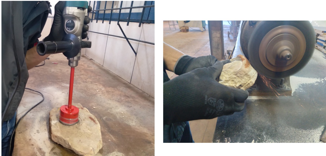
Figure 2.12: First attempt at molding the specimen.
