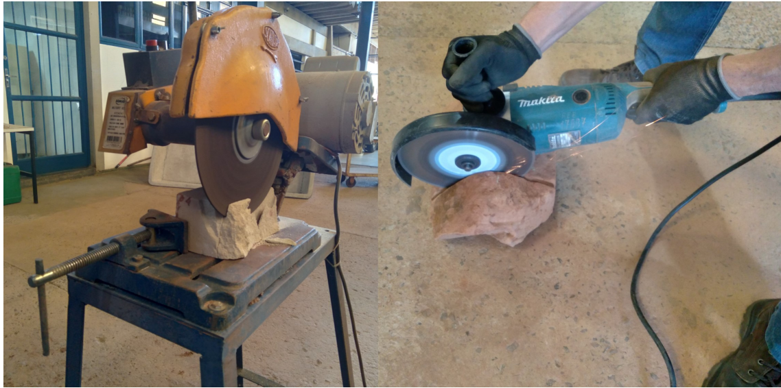
Figure 2.15: Cutting the samples with a circular saw to prepare them for another configuration with enough spindle stroke to remove the specimens.
