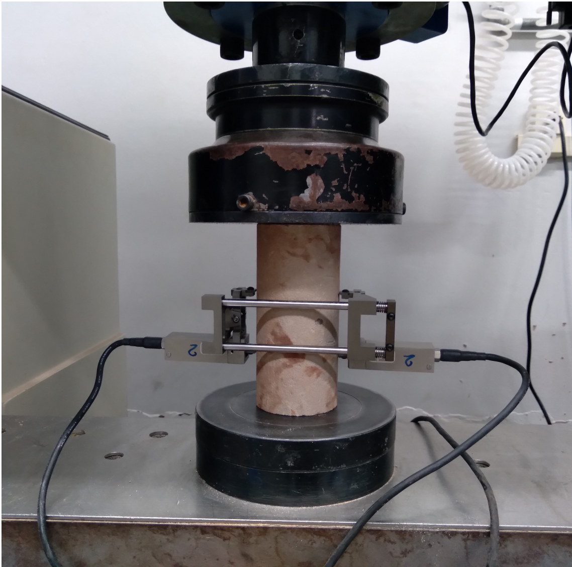
Figure 2.24: Test layout to obtain Young's modulus.
