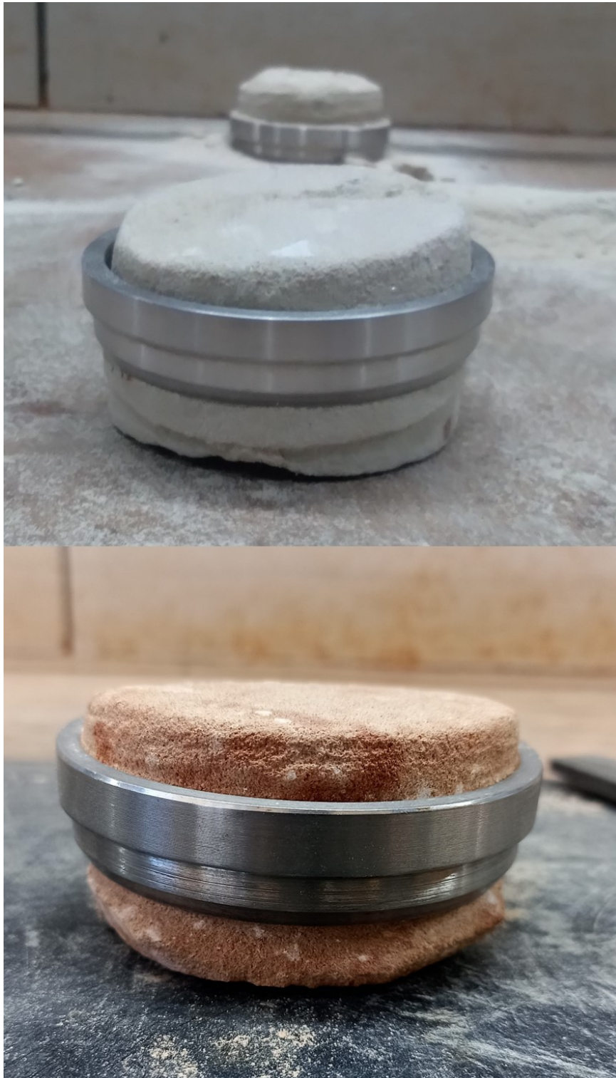
Figure 2.31: Gray and brown sandstone samples in the molds for oedometer testing before grinding the top and bottom.
