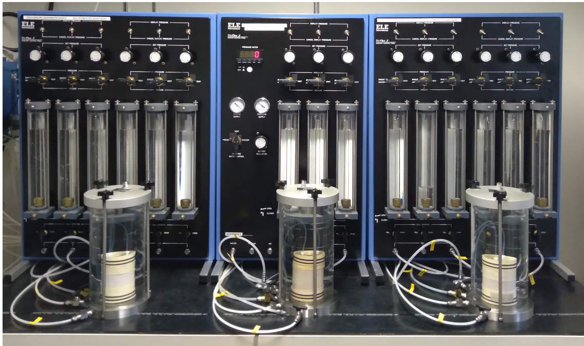
Figure 2.35: Flexible wall permeameter running three tests.
