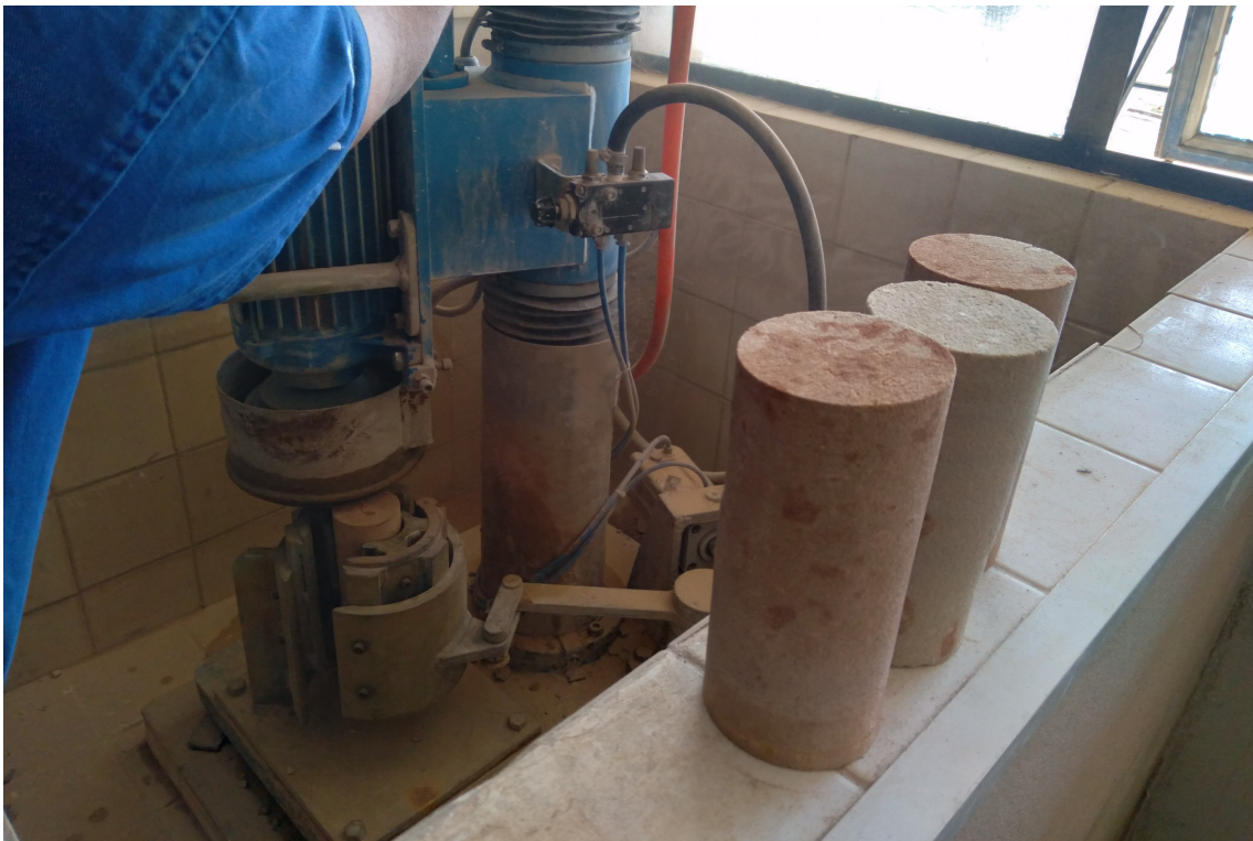
Figure 3.8: The specimen grinding machine polishes the top and bottom of sandstone samples.
