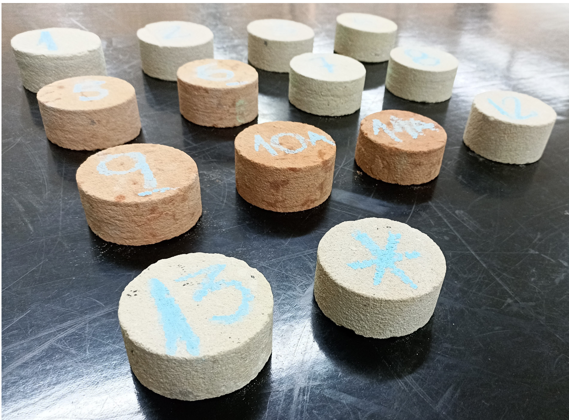
Figure 2.26: Specimens suitable for the diametrical compression test as recommended by ASTM D3967 (2016).
