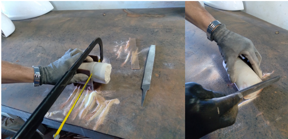
Figure 2.19: Specimen's top and bottom preparation by removing the coarse layer.
