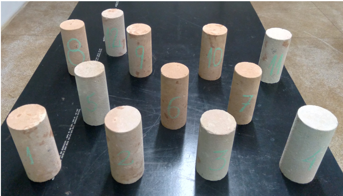
Figure 2.21: Sandstone specimens completed and identified for testing.
