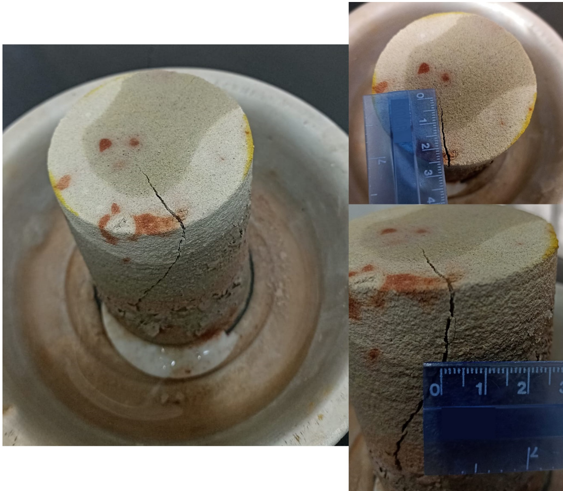
Figure 2.62: Fracture in a gray sandstone sample caused by the expansion of the material exposed to saturation by capillarity.
