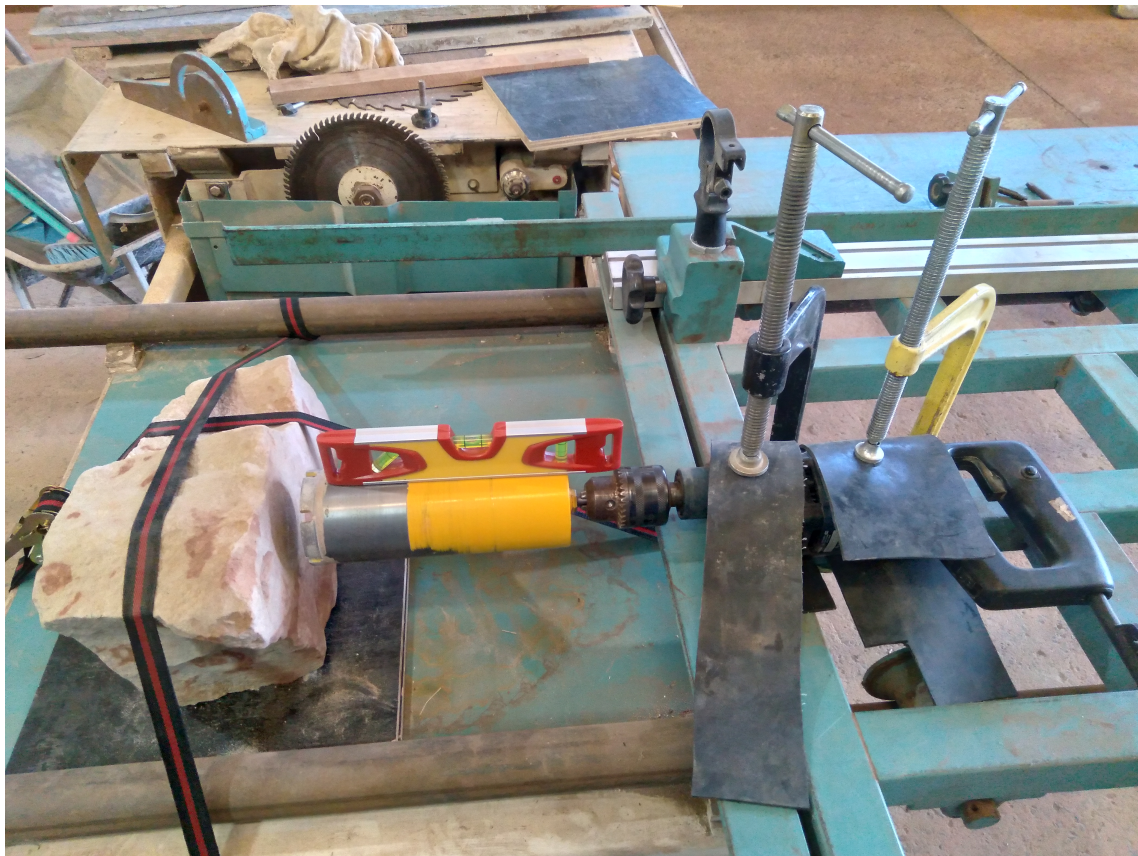
Figure 2.16: Final setting with a diamond hollow core drill adapted to have enough stroke to remove the sandstone specimens.
