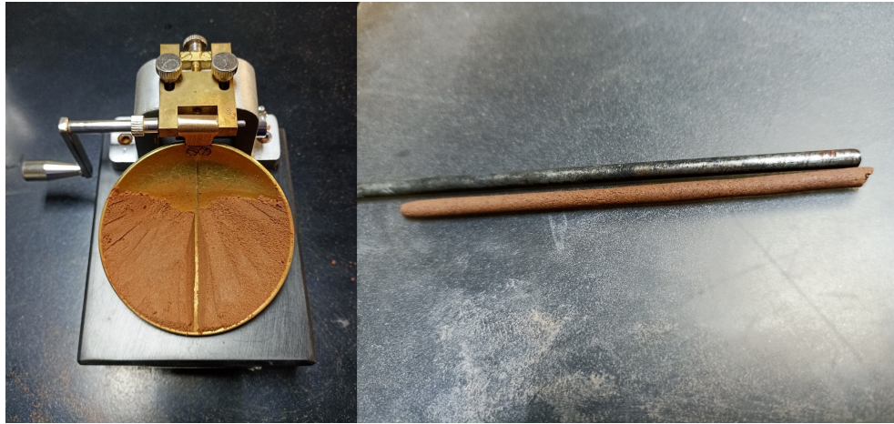
Figure 2.10: Liquidity and plasticity limits exemplified by the brown sandstone sample
