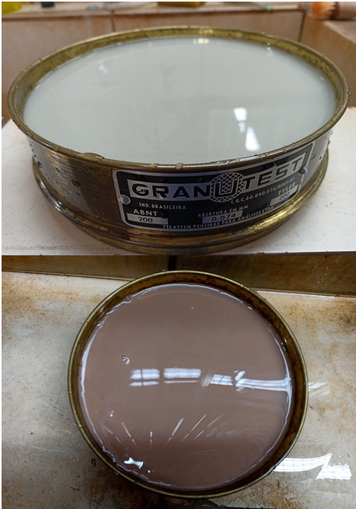
Figure 2.9: Washing the material to be sieved. Despite having few fines, the sandstone could retain water on the 0.075 mm sieve.
