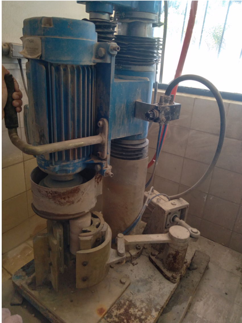
Figure 2.20: Fine polishing of sandstone rock sample using the specimen grinding machine.
