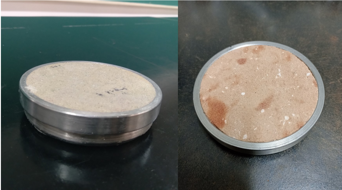
Figure 2.32: Gray and brown sandstone ready for the oedometer test
