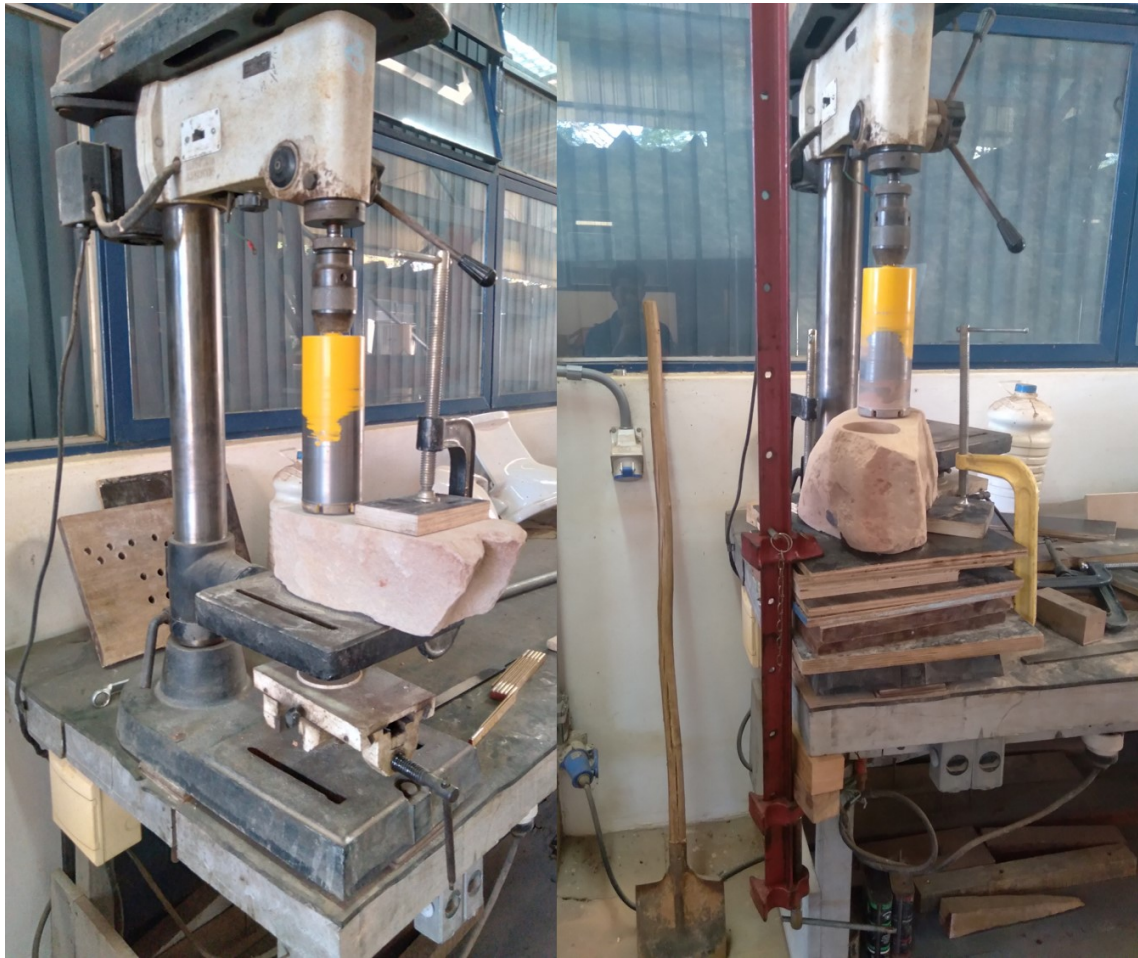
Figure 2.14: Bench drill proved helpful, but there was a short spindle stroke when removing the specimens.
