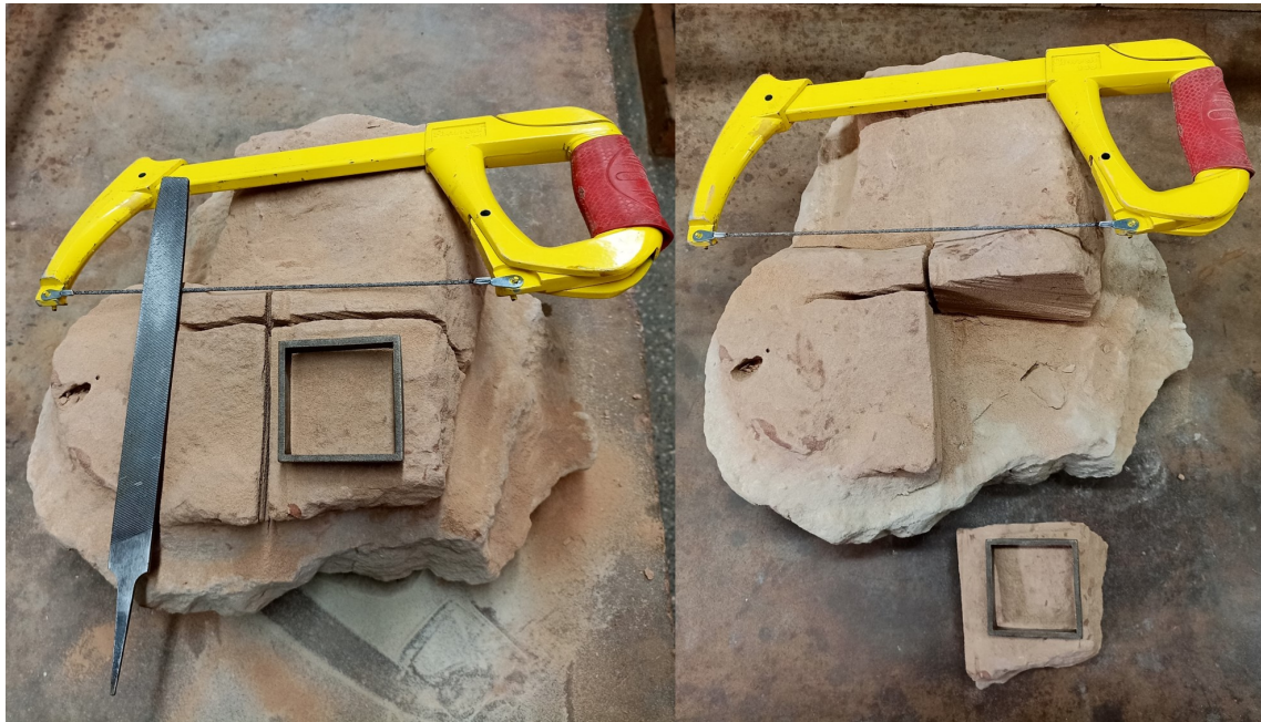
Figure 2.27: Molding of the specimens for the direct shear tests.
