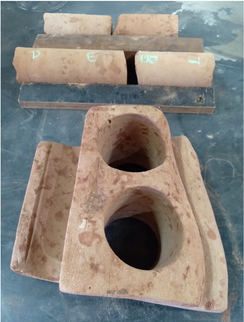
Figure 2.17: Longitudinal and transverse core samples.
