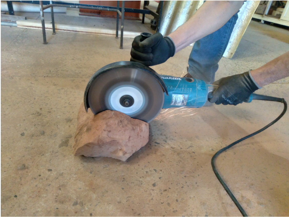
Figure 3.6: Sandstone sample cutting process.
