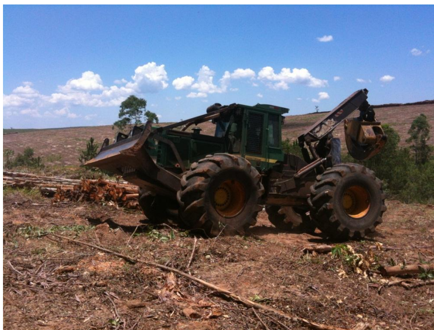
Figura 4. Trator florestal Skidder John Deere, modelo 848H.
