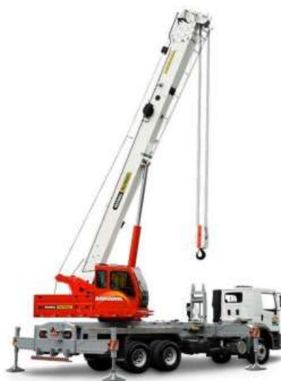
Figura 2 – Truck crane (TC).
