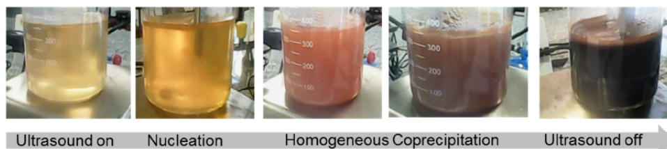
Figure 1. Changes in the solution color during ultrasonic cavitation: nucleation and homogeneous coprecipitation.
