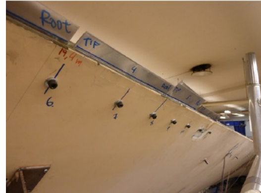
(b) Damage bolted to control the damage size and any additional anomalies introduced by the impact that generates the damage.
