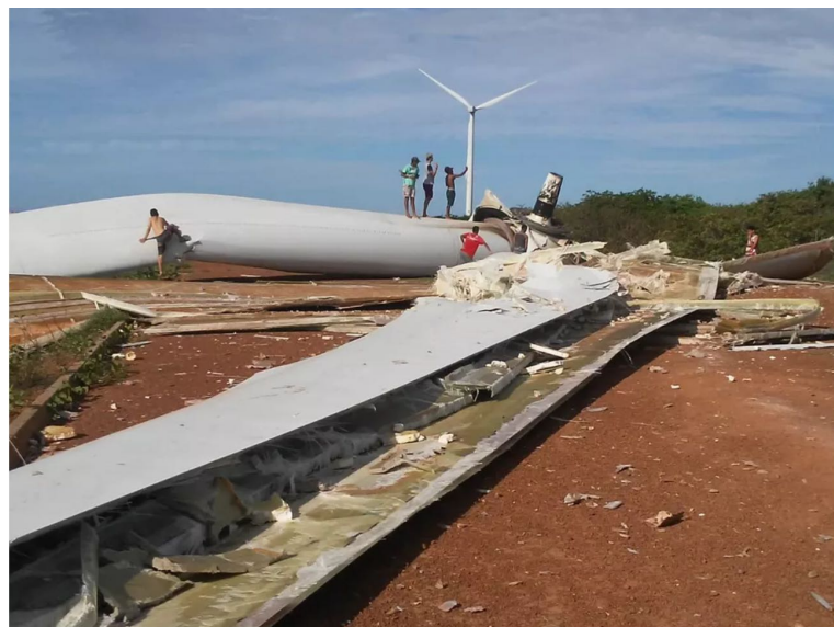
Figure 1: Accident in which a wind turbine's blades came off, on the coast of Piauí - Brazil.
