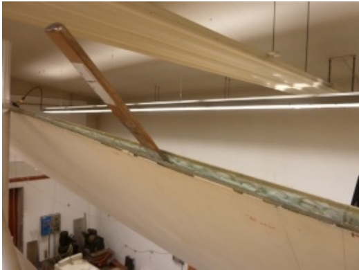
(a) Damage introduced by chisel in the trailing edge.
