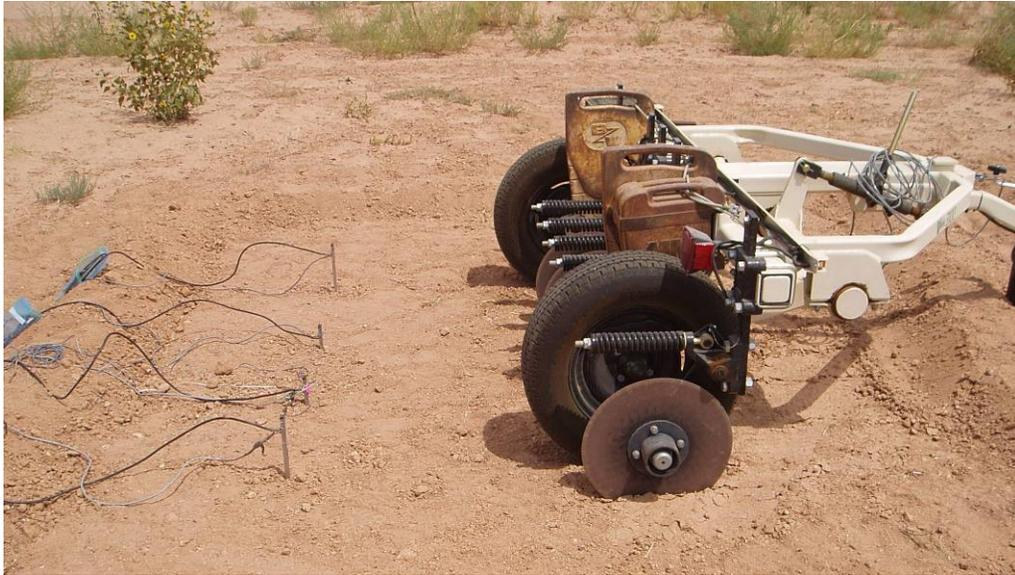
Figure 3. Set up of the Veris 3100 sensor for static measurements of ECa. On the left side of the picture are shown a set of four TDR probes for measurement of moisture content.
