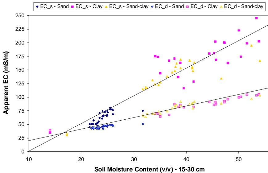
Figure 6. Effect of soil moisture content on the Veris 3100 output in three locations of different soil textural characteristics.
