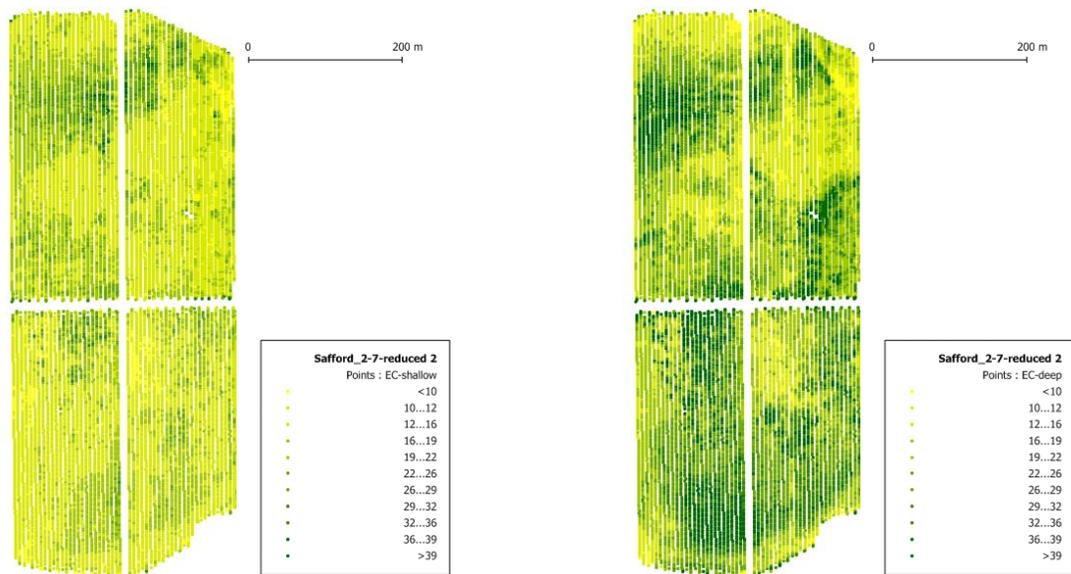
Figure 4. Maps showing spatial variability of ECa in a field near Safford AZ. Map on the left corresponds to the shallow depth (0-30 cm); the map on the right is the deeper reading (0-1 m).
