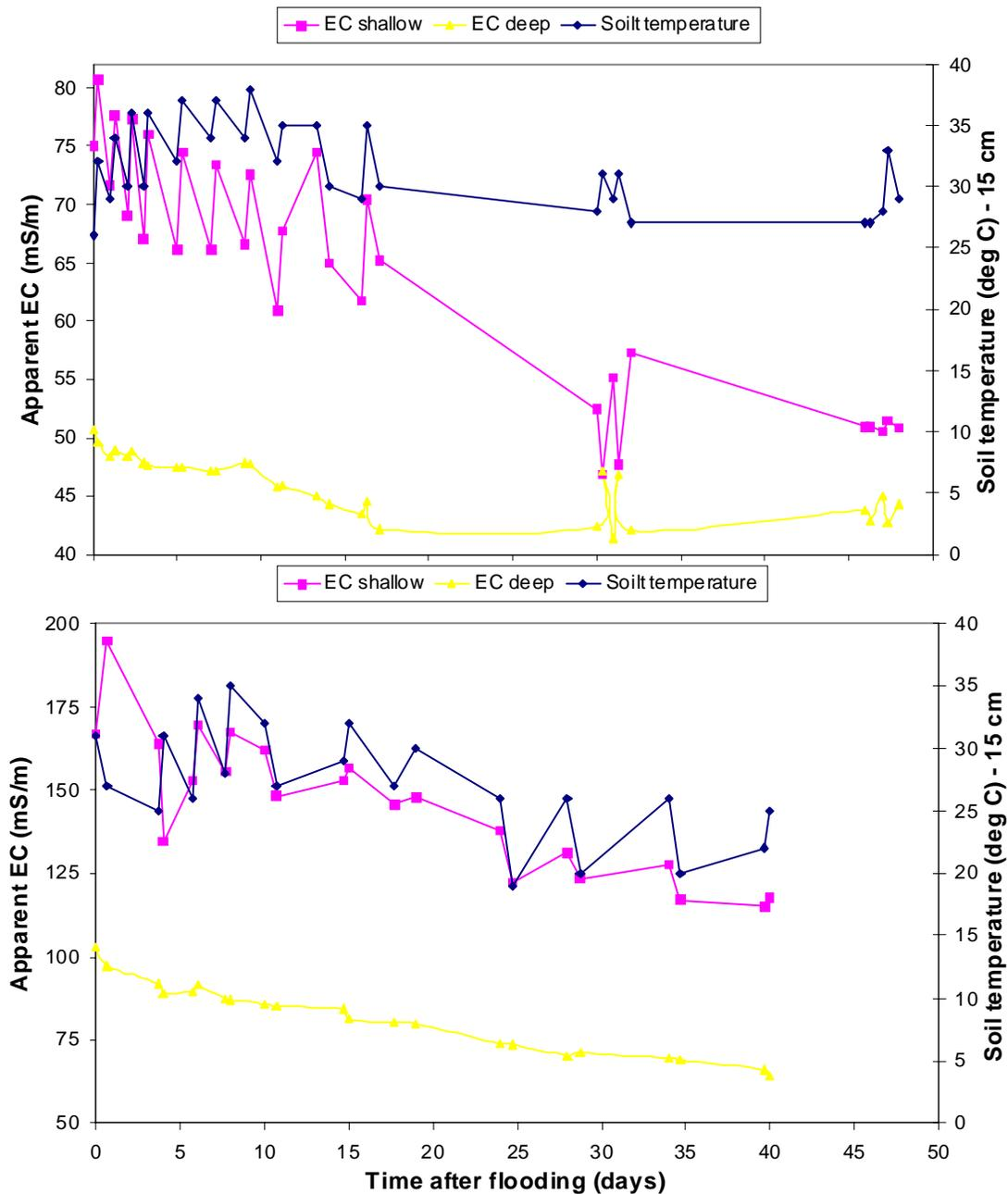
Figure 5. Times-series plots showing fluctuations of ECa due to soil temperature and time elapsed after flooded irrigation. Plot on top corresponds to the site with Sandy clay loam texture; meanwhile the bottom plot corresponds to a location with Sandy clay texture.
