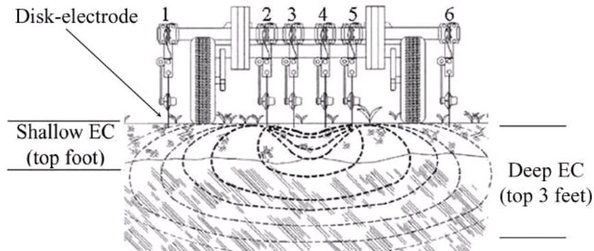
Figure 1. Drawing of the Veris 3100 showing the trailer cart frame and wheels, and the disc electrodes (1-6). The system acquires two signals simultaneously at different depths.
