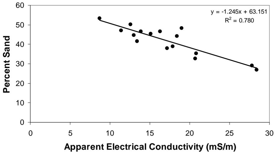
Figure 5. Linear regression plot of ECa generated with the Veris 3100 and percent sand values determined with laboratory techniques.
