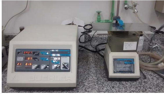
(a) Buehler® Electromet 4 electrolytic polisher composed of an electric circuit and an acid solution pump capable to produce controlled mass loss.
