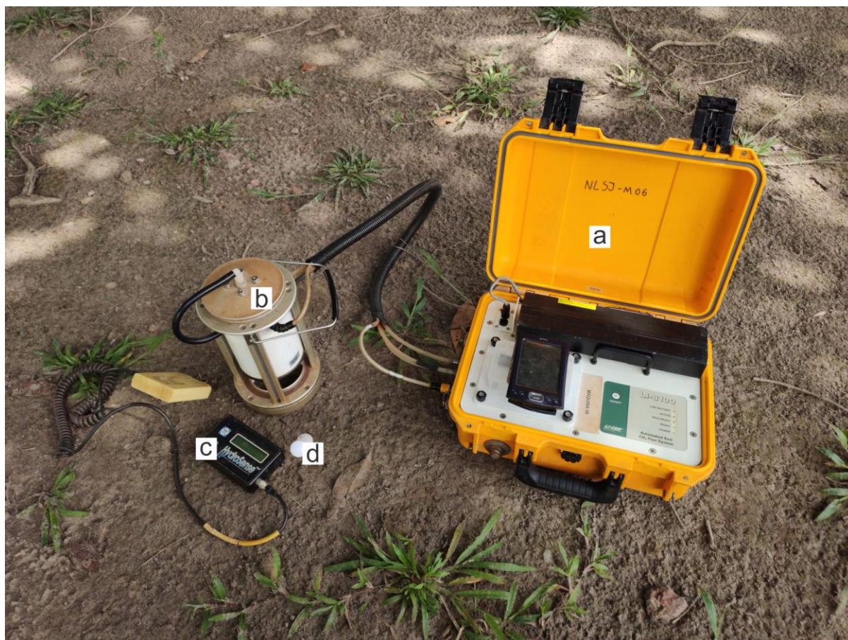
Figure 3. LI-COR model LI-8100 portable system (a) connected to the soil chamber (b), soil moisture sensor (c) and soil temperature sensor (d).
