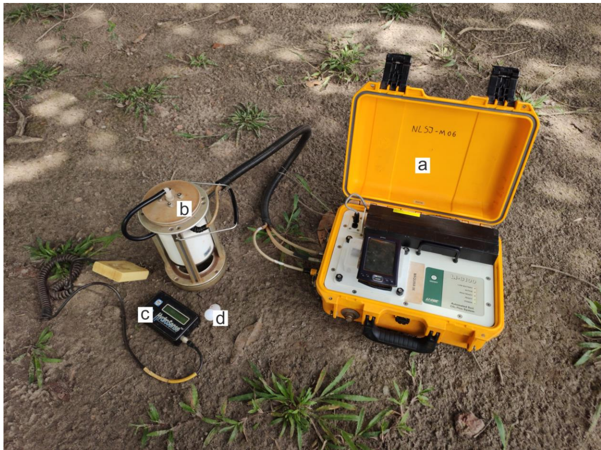
Figure 2. LI-COR model LI-8100 portable system (a) connected to the soil chamber (b), soil moisture sensor (c) and soil temperature sensor (d).
