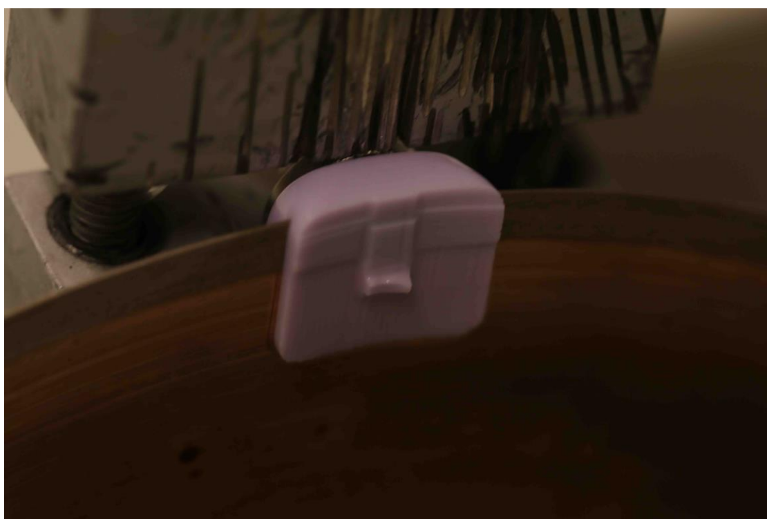
Figure 1 – CAD/CAM blocks with approximate width of 0.6 mm.
