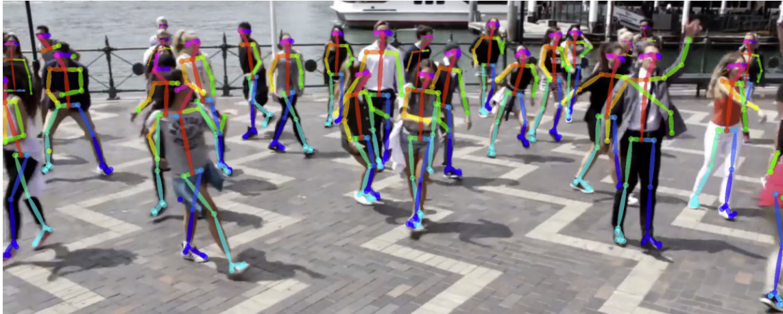
Figure 2 – 2D human poses estimated in an image and represented through the COCO model (LIN et al., 2014).
