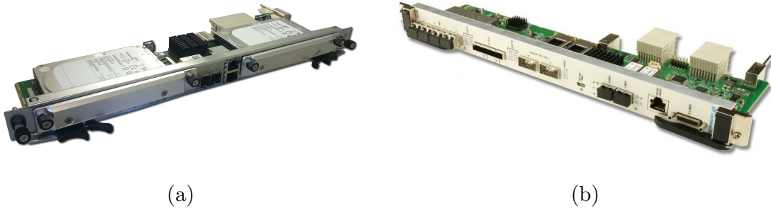
Figure 4: RTM for AdvancedTCA blades. (a) is the RTM436 from SANBlaze and (b) is the ART132 from Vadatech.
