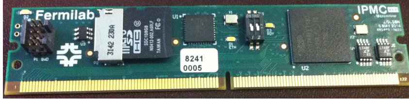
Figure 14: Picture of the Pulsar I Ib IPMC card designed by Fermilab and the central element of this project.
