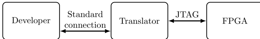
Figure 8: Diagram representing the connection between developer and FPGA during the development stage, from any standard interface to a JTAG connection.
