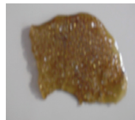
Figure 4 - Initial results of the dissolution of EPS with d-limonene
