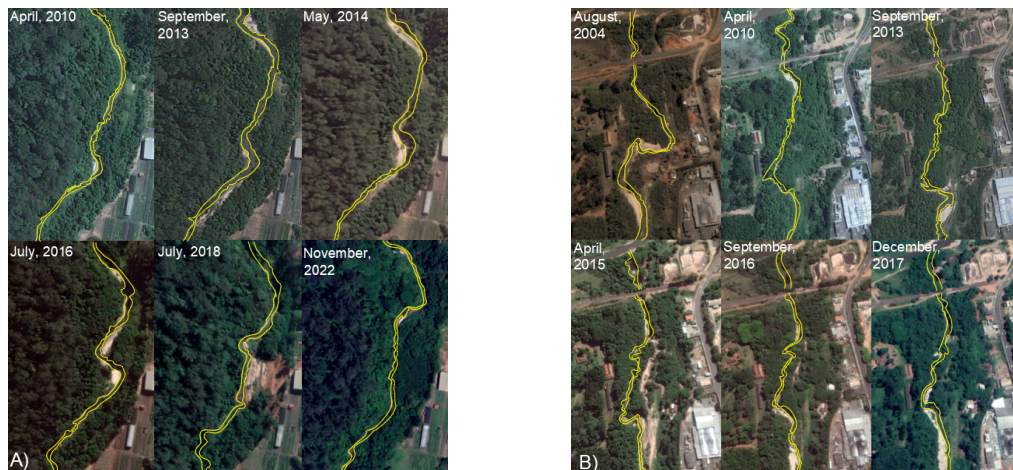
Figure 2-4: Delineation of changes in the banks of two stretches (A and B) near the outlet of the stream between 2004 and 2022
