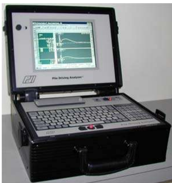
Figura 9 - Pile Driving Analyser (PDA)
