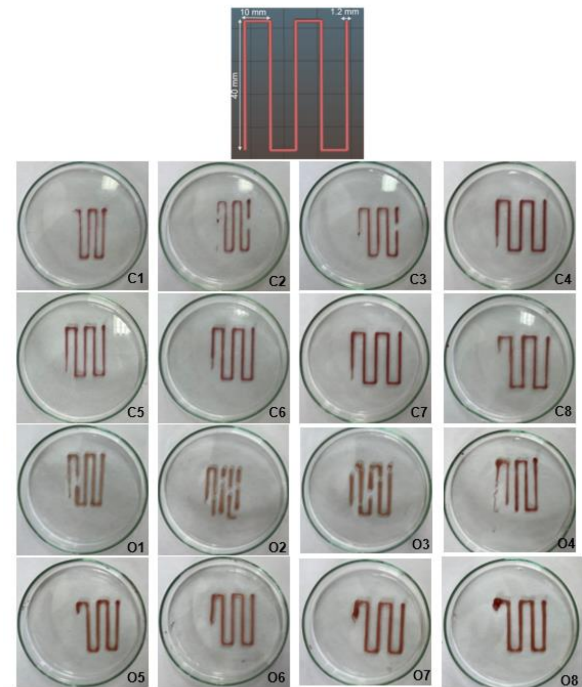
Fig. 6 - Strand thickness analysis: Printed strands, designed with specific length and width parameters (on the top of the figure) and measured using ImageJ. The numerical annotations correspond to the associated printing parameters. "C" denotes the commercial sodium alginate-based ink, while "O" represents the ozonized sodium alginate hydrogel, both pre-crosslinked with \text{CaCl}_2 (25mM), incorporating agar and encapsulating an anthocyanin-rich extract
