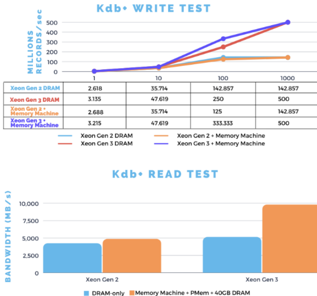
Figure 2 – Read and write benchmark of 1st and 2nd generation of Intel Optane PM DC, comparing DRAM performance with DRAM+DCPMM in each platform in a database workload using KX's kdb+.
